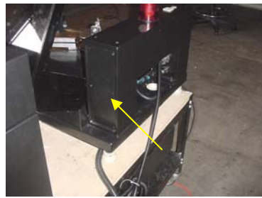
Open the back cover on X-Ray tube chamber from back of machine
