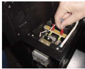
Plug in two wires from light into holder in
