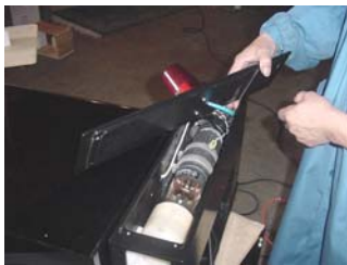
Open the top cover on X-Ray machine; tighten the Indication light from back of cover
